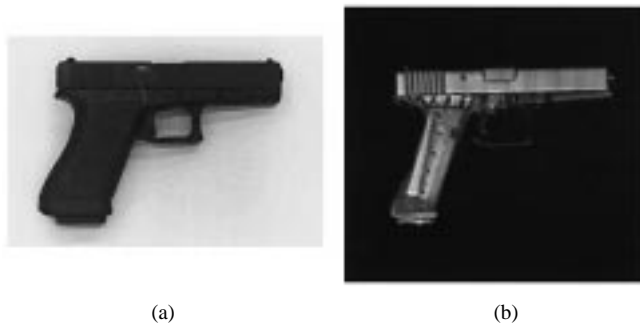
Fig. 7. (a) Optical image and (b) 100–112-GHz wide-band holographic image of a Glock-17 handgun.
