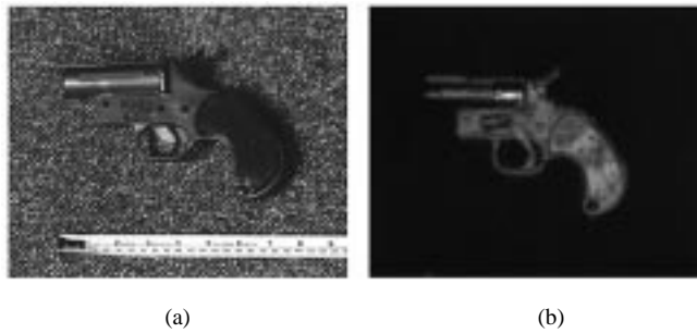
Fig. 8. (a) Optical image and (b) 100–112-GHz wide-band holographic image of an Olin plastic flare gun.
